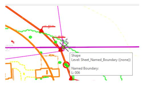
E. Select **Modify Element** and click on the adjacent point on the **006** Named to the left (inside) of the intersection point and place it on the bottom right corner of **030**.
