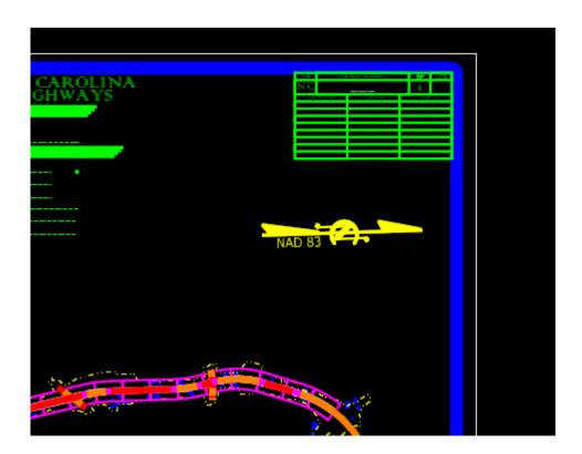
I. Use the Microstation **Edit Data Field** command to enter the **Scales** and **DESIGN DATA** values.
